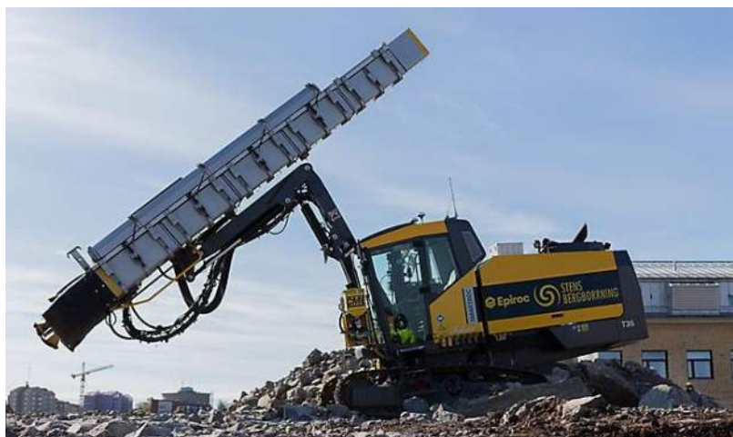
Figure 6.2 Epiroc Smartroc T40 drill with noise mitigation package (Image source: Epiroc Website)
