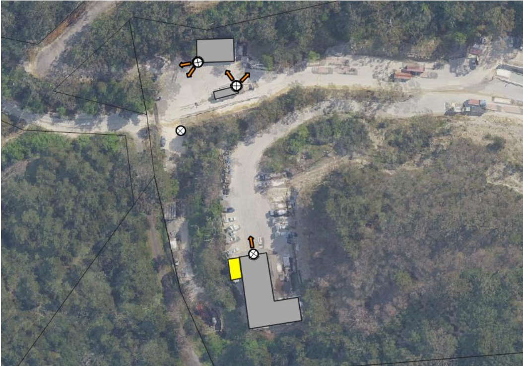
Figure 3.1 Site lighting – Site office, weighbridge and transport area
