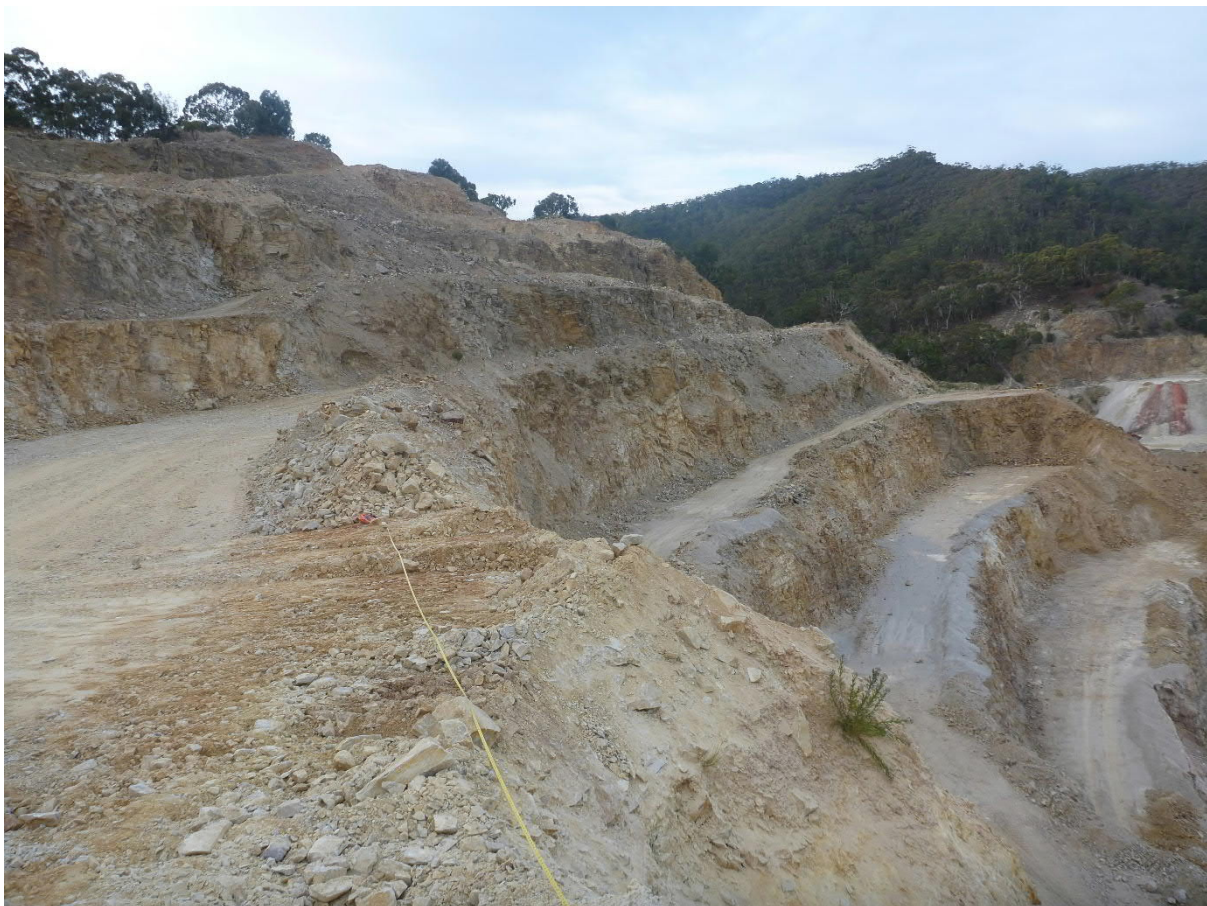
Plate 7: The eastern highwall in section is a bedded moderate strength metamorphosed rock mass which while jointed perform well in service as is clearly evident in this image. Bedding is sub horizontal and the rock mass is not folded to any significant degree. Minor warping of the bedding planes and small scale fault displacements are also recognised in this wall.
