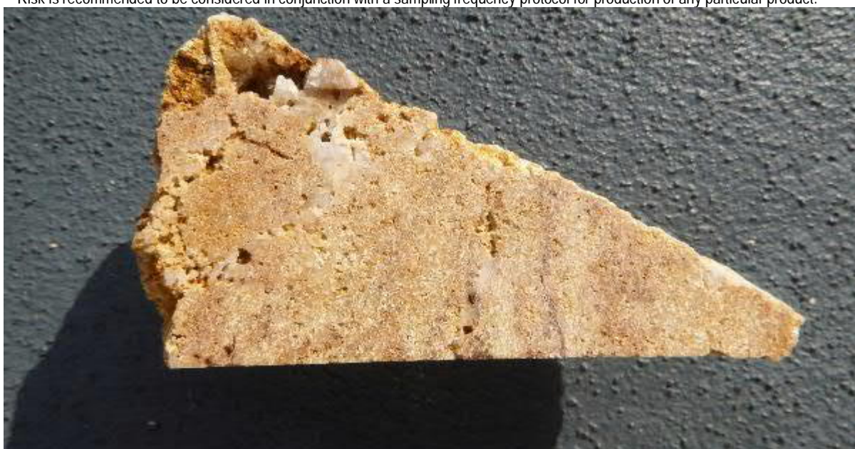
Plate 1: Photograph displaying sectioned face of the quartzite including medium and coarse grain size of constituent quartz and feldspar as well as a pervasive network of ferruginous veins and associated weathered voids.
