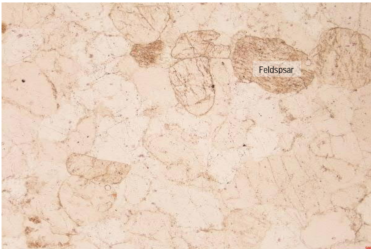
Plate 3: Microphotograph utilising plane polarised light to better distinguish dusty feldspar profiles from clear quartz and illustrate calcite, opaque and rare zircon distributions within the quartzite.
